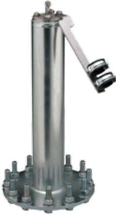
A probe installed in a flanged pipe for external mounting, for example on a flue duct. This probe is used when an extractive probe may not be used directly in the process to be analysed.
