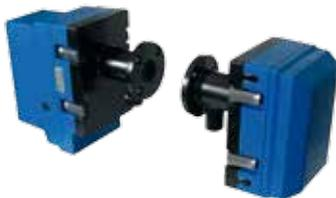
Continuous measurement of opacity and dust concentration with low detection limits. The monitor uses the transmission measuring principle and is mounted cross-stack. The monitor is approved in accordance with US legislation (EPA) and is suitability tested by TÜV.
