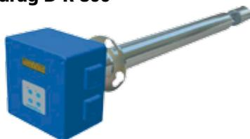
Continuous measurement of dust concentration with low to medium detection limits. The monitor uses the reflection principle and is based on innovative laser technology that enables simple flange mounting. The dust monitor complies with European regulations (EN14181) and is approved by TÜV.
