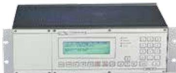
A TOC analyser, which is available as a 19" rack model or as an integrated analyser with a heated probe for mounting directly onto the flue duct.
