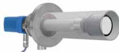
Continuous measurement of flow. The monitor uses ultrasonic measurement. Because the transmitter and receiver are mounted across the flue-gas duct, a measurement can represent the entire cross-section. Approved in accordance with EN15267-3 and approved by TÜV.
