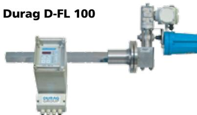
Continuous measurement of flow, using the differential pressure principle. Because the meter can be configured with a length of up to 8 m, a measurement can represent the entire cross section of most flues.
